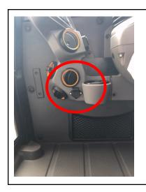
1 x 12V, 25 Ampere 3 Pin plug for joystick control box.
